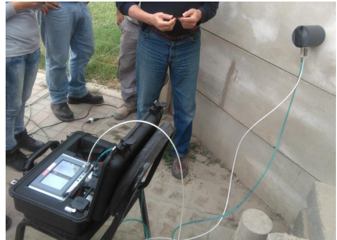
Fig. A.1 - Aspect of the vacuum cell's concentric rings (l.) and cell applied on a vertical surface (r.)
